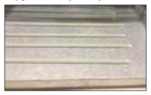
Figure 3.4: GFRP Bars Exposed to the Alkaline Environment
