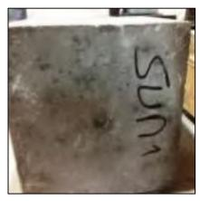
Figure 5.1: Complete Pullout Failure
