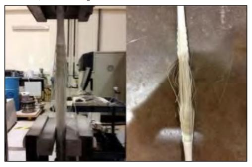
Figure 5.9: GFRP Bar Mode of Failure after a Tensile Test
