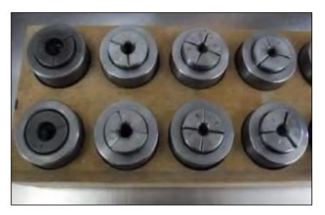
Figure 4.8: Steel Grips for Gripping Both Ends of GFRP Bars during the Uniaxial Test
