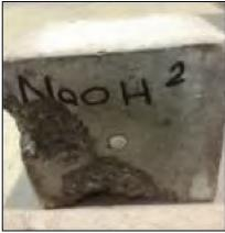
Figure 5.3: Concrete Block Split
