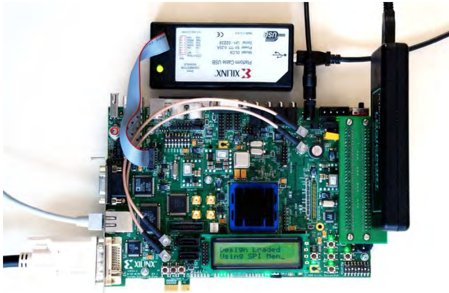
Figure 47: ML505 Evaluation Board [53]
