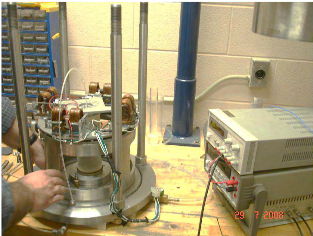
Figure 2.1: Specimen preparation in a resonant column device
