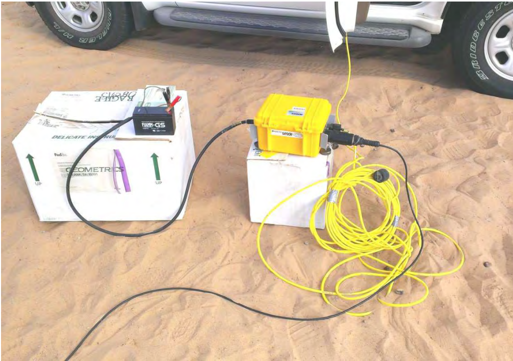
Figure D5: Setting up geode with the power supply and spread cable on Site S14
