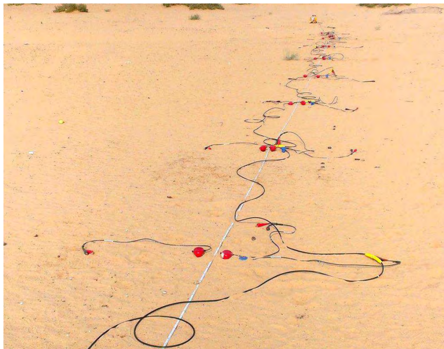
Figure D4: A view of horizontal and vertical geophone lines on Site S13
