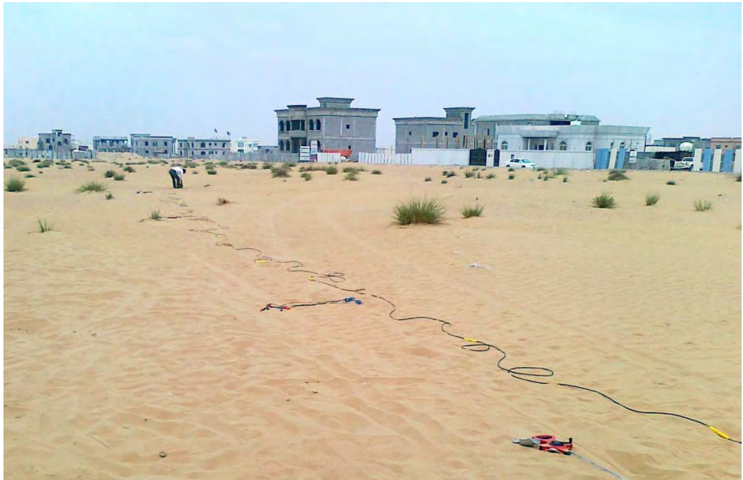
Figure D1: Spreading the cable on site S12
