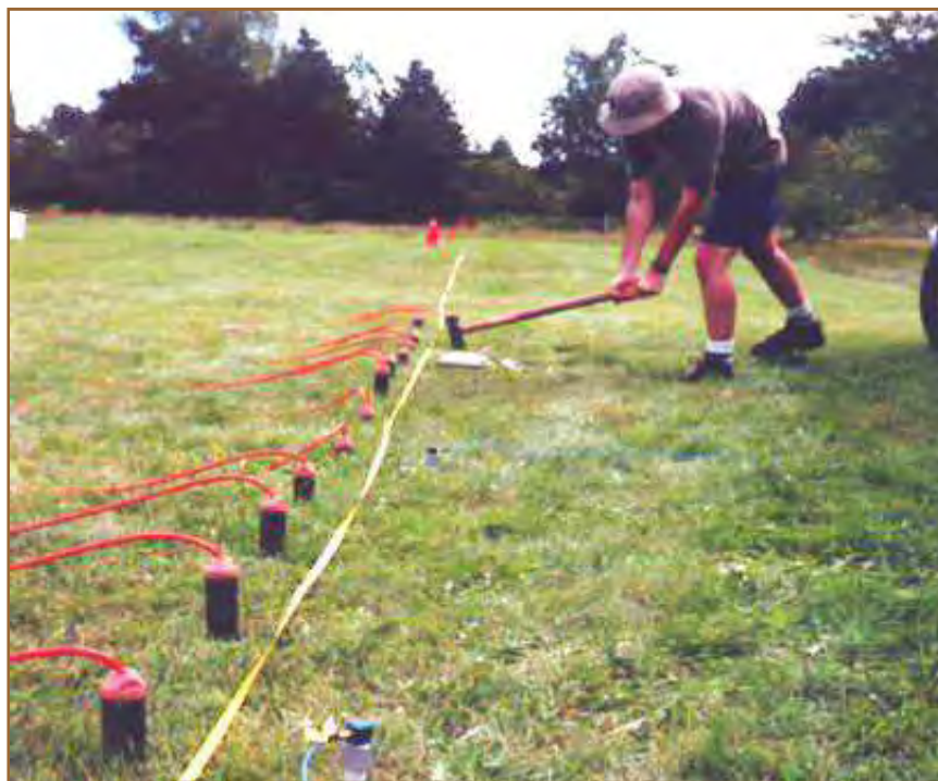
Figure 2.11: Typical test setup and wave generation during seismic testing in the field
