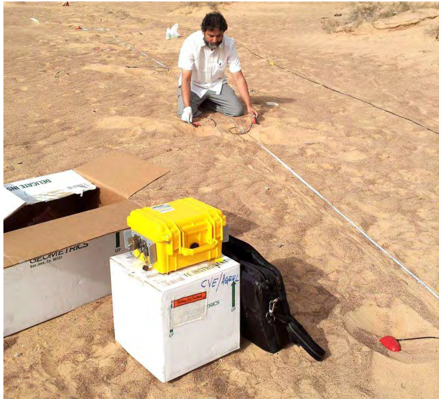
Figure D3: Inserting geophones at predetermined locations on Site S10
