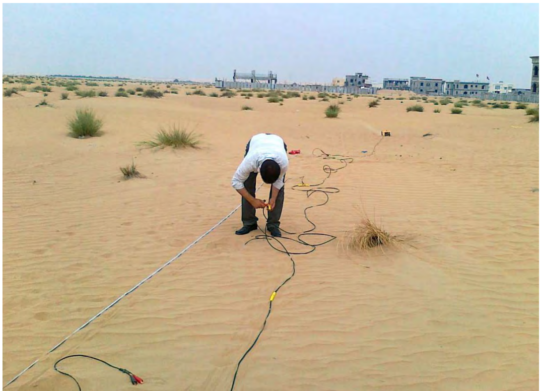
Figure D2: Connecting geophones to the spread cable on Site S12
