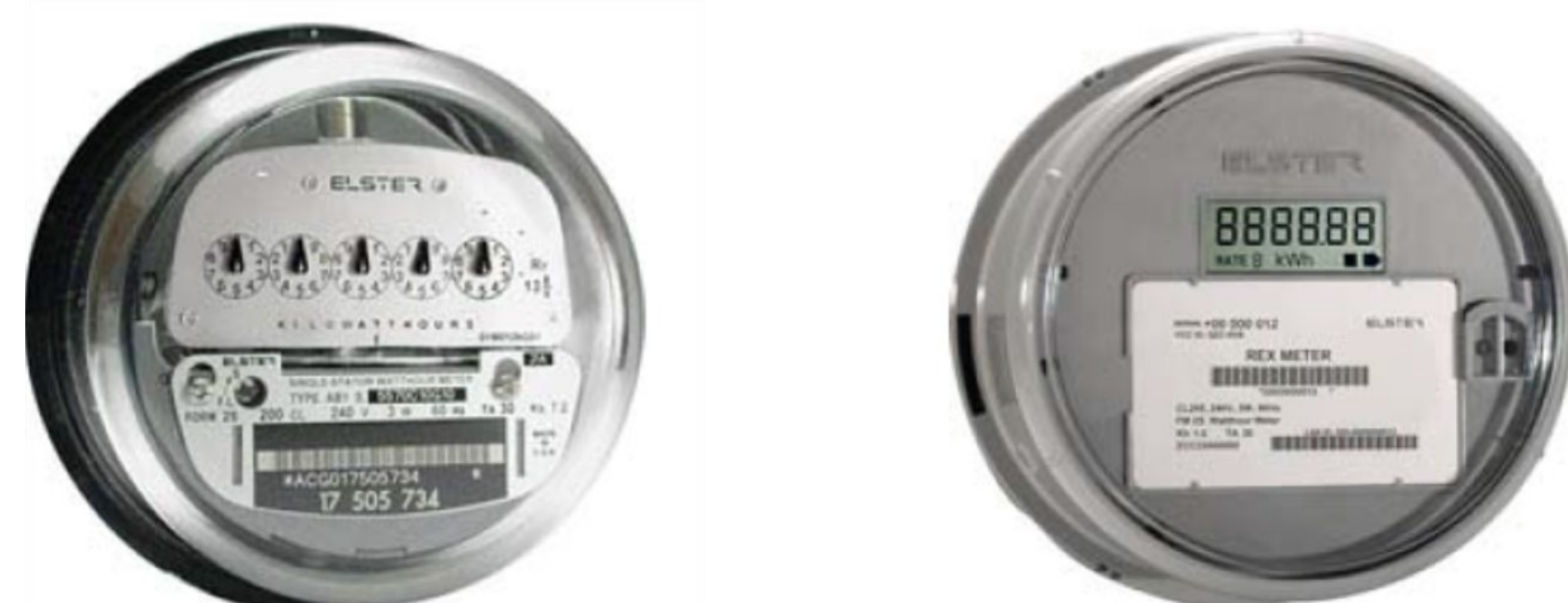
Figure 2: Conventional meter on the left and a smart meter on the right [2]
