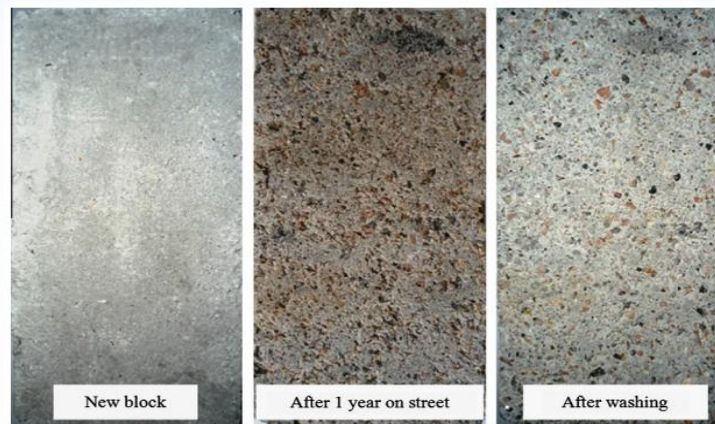
Figure 3: Nano coating of concrete [10].
