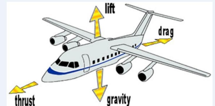
Figure 4: Forces on an aircraft [10]
