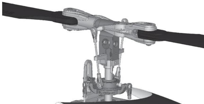
Figure 6 : Flybarless Helicopter Rotor Head [49]
