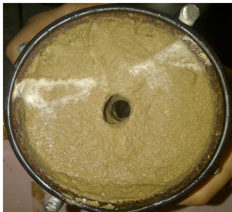
Figure 3.4: Prepared test specimen (hole diameter at the end of the test)
