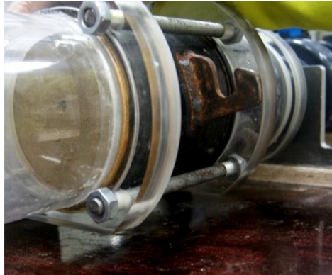
Figure 3.3: Specimen during the test (hole diameter at time zero)
