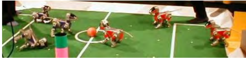
Figure 3: Particle filters have been used successfully for on-board localization of soccer-playing Aibo robots with as few as 50 particles [47].
