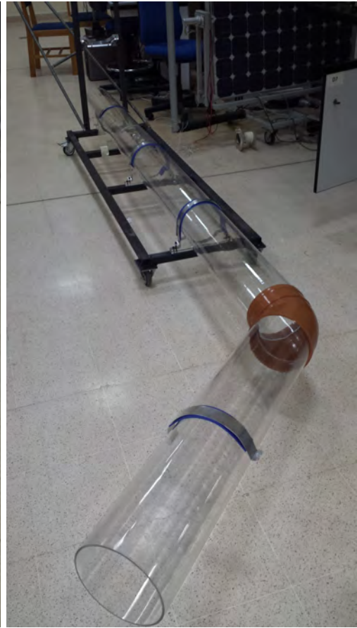
(b) Straight pipe with one elbow.
