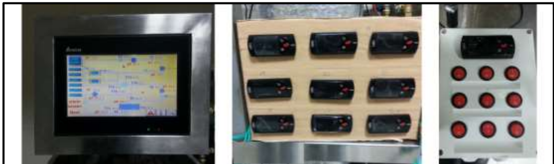
Figure 64: Experimental data measurements system including 12 channels for temperature reading, 8 channels for pressure reading
