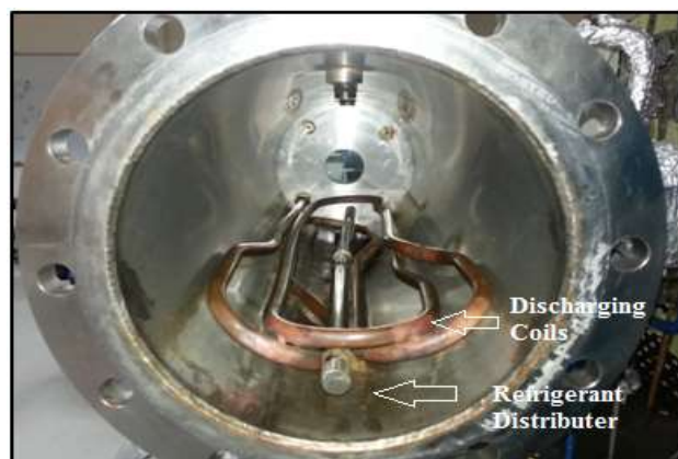
Figure 16: Refrigerant distributor inside the direct storage tank
