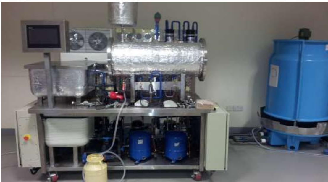
Figure 12: Picture view of the experimental direct thermal energy storage test rig
