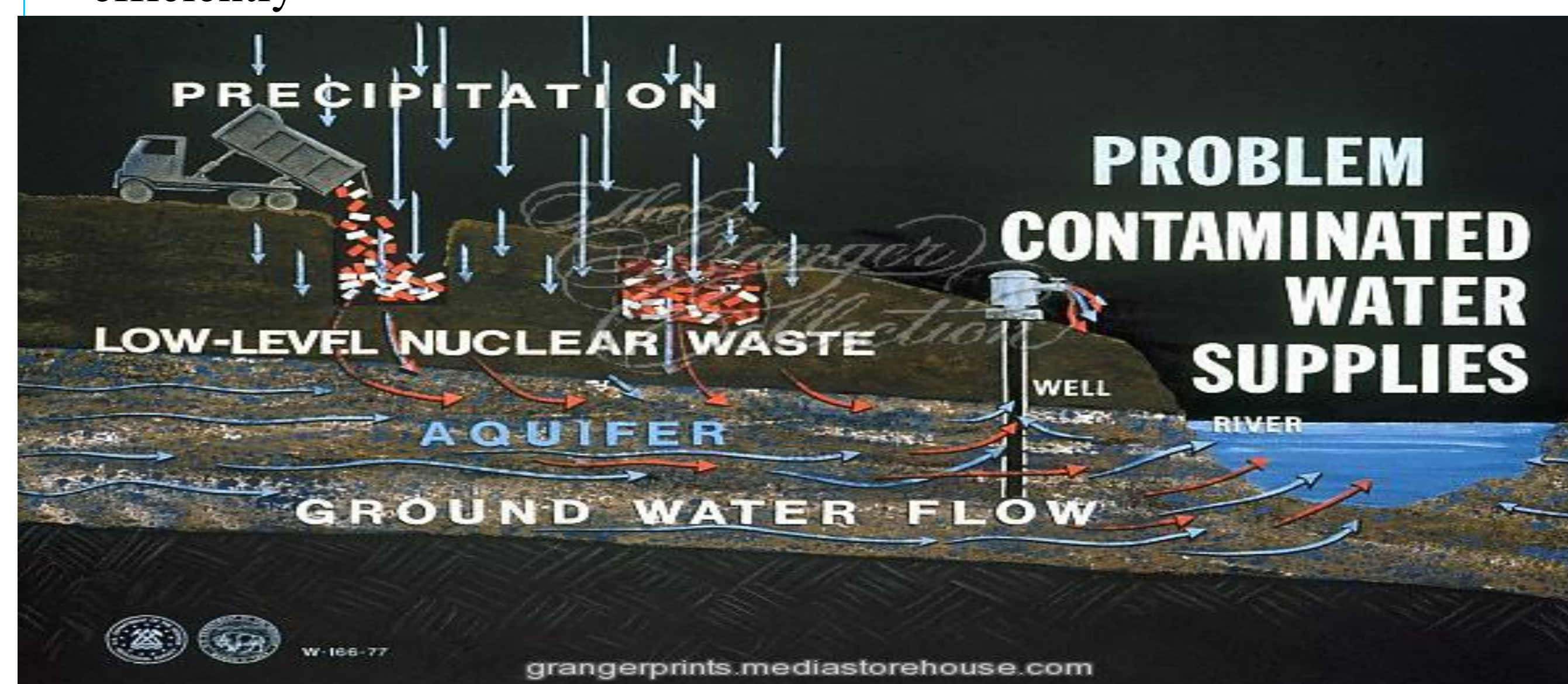
Figure 2: Illustration of How LLW May Contaminate Water Sources [3]
