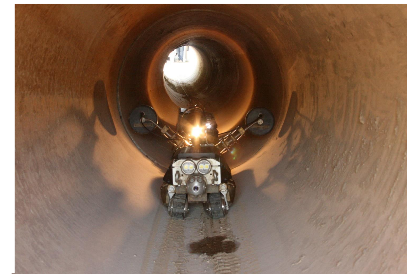
Figure 4: Evaluation Robot inside Pipeline [8].
