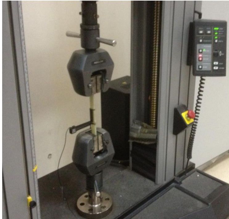
Figure 25 Specimen during tensile stress testing
