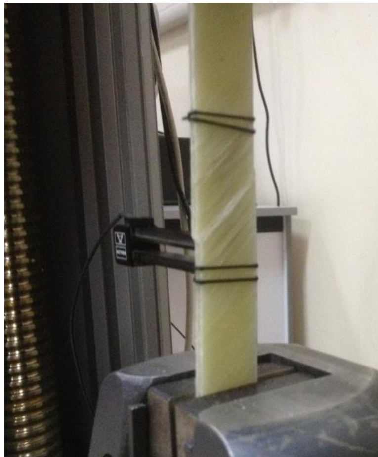
Figure 26 Example of a 45° specimen after failure
