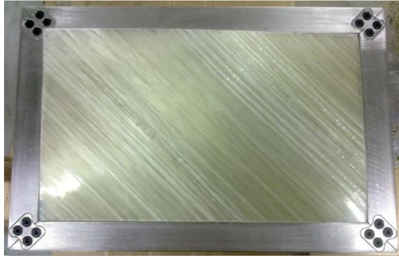
Figure 13 Aluminum mold with the prepreg laminas
