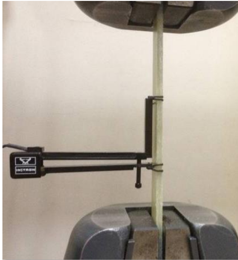
Figure 24 Specimen with extensometer
