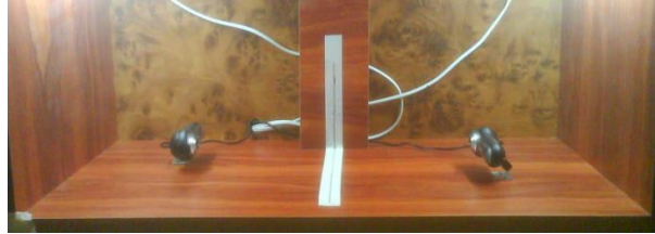
(a) Data collection box fixed with two cameras to capture hand images
