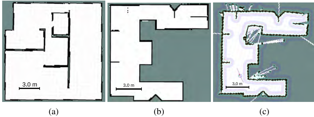
Figure 37: Occupancy grid maps generated using the proposed exploration strategy, single robot case.
