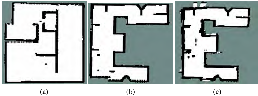
Figure 38: Occupancy grid maps generated using the proposed exploration strategy, three robots case.
