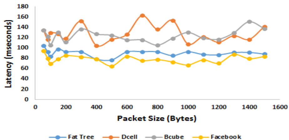
Figure 5.2 Latency comparison for the standard topologies with different packet size (All-to-All traffic)
