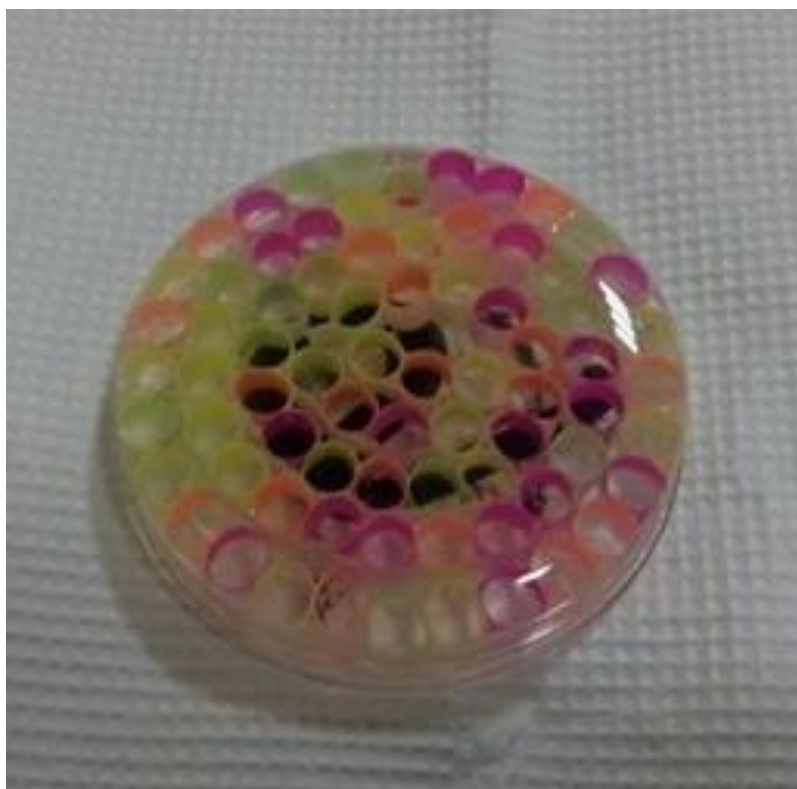
Figure 4.1: Casting mold of hydrogel on straws.
