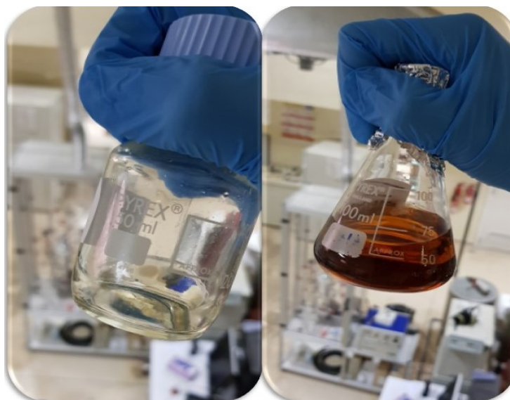
Figure 18: Color change of [EMIM][OAc]. Image on the left is for new [EMIM][OAc], while the image on the right is for [EMIM][OAc] solution after boiling for long time
