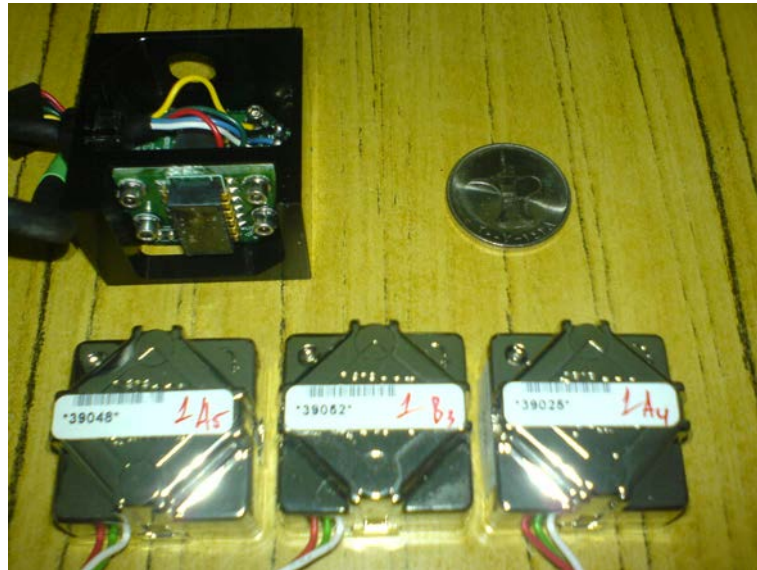
Figure 4.31: Sensors utilized in this thesis. In the upper left corner appear two dual-axis accelerometers ( \pm 4g each) and below appear three single-axis gyroscopes ( \pm 100^\circ/h each).
