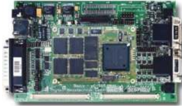
Figure 2-20: phyCORE-MPC565 Development board
