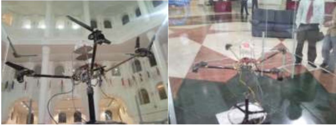
Figure 2-30: Different Views of the 4DOF Test Stand
