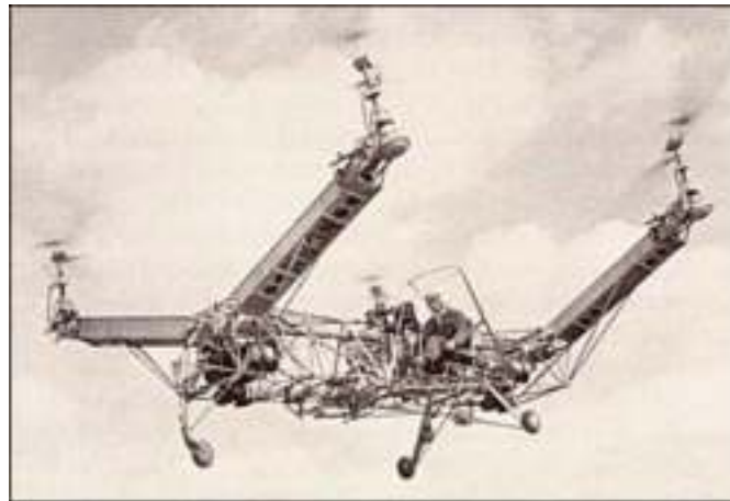
Figure 1-5: Convertawings Model "A" Quadrotor
