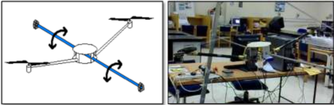
Figure 2-29: 1-DOF Test Stand
