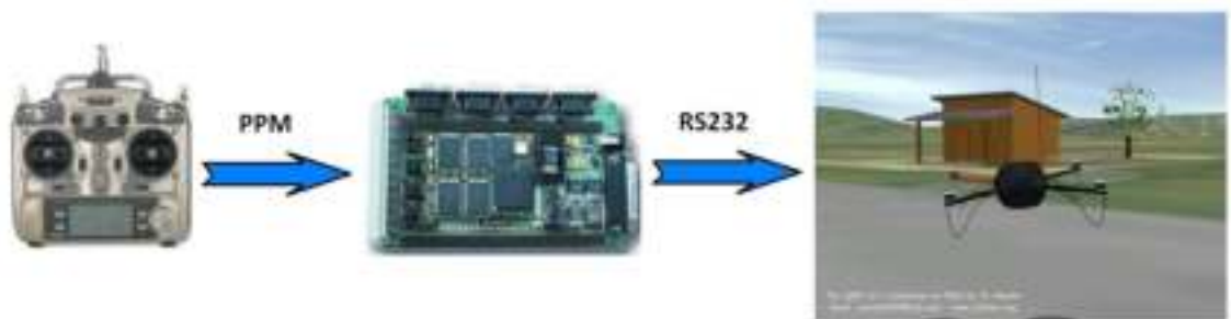
Figure 2-27: Decoding Process of the PPM Signal
