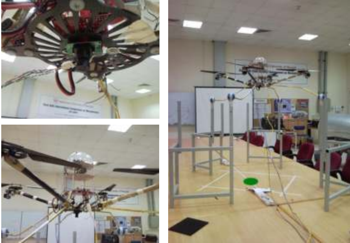
Figure 2-25: CMUcam3 fixture on the AUS quadrotor
