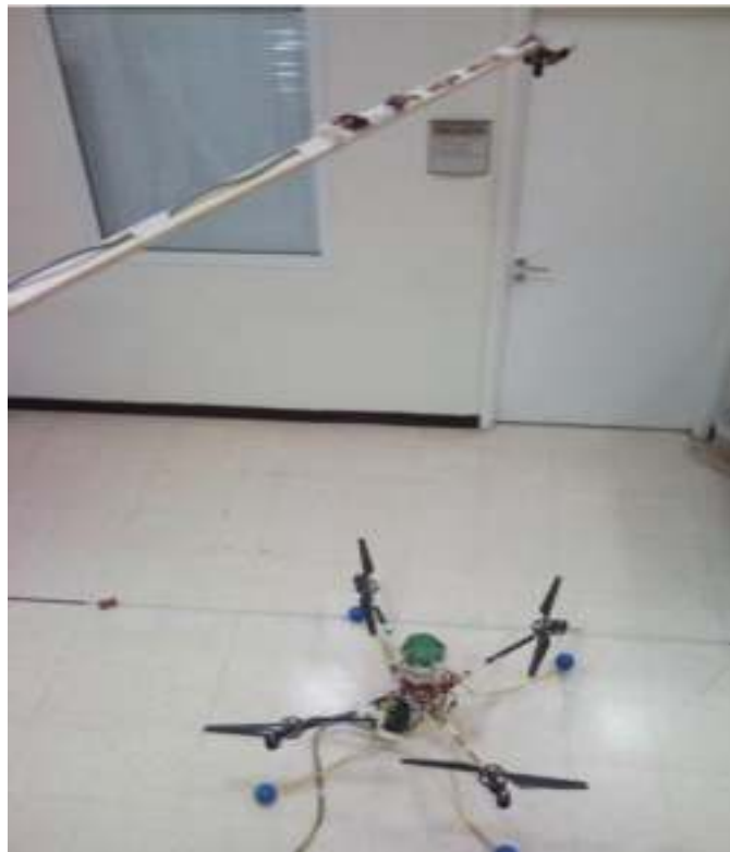
Figure 2-22: CMUcam3 setup to track the green dome of the AUS quadrotor
