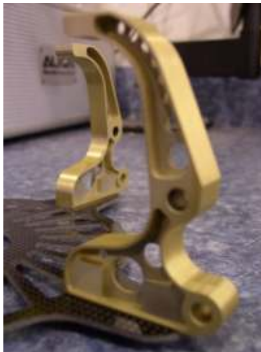
Figure 2-5: Risers fixed on the base plate.
