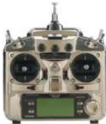
Figure 2-10: Futaba RC Transmitter
