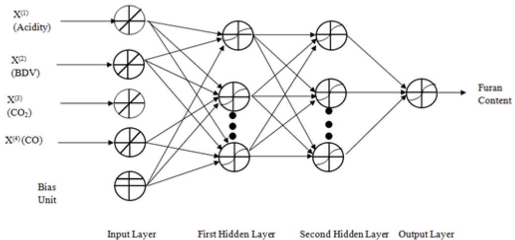
Figure 4 Artificial neural network structure used for prediction of furan content
