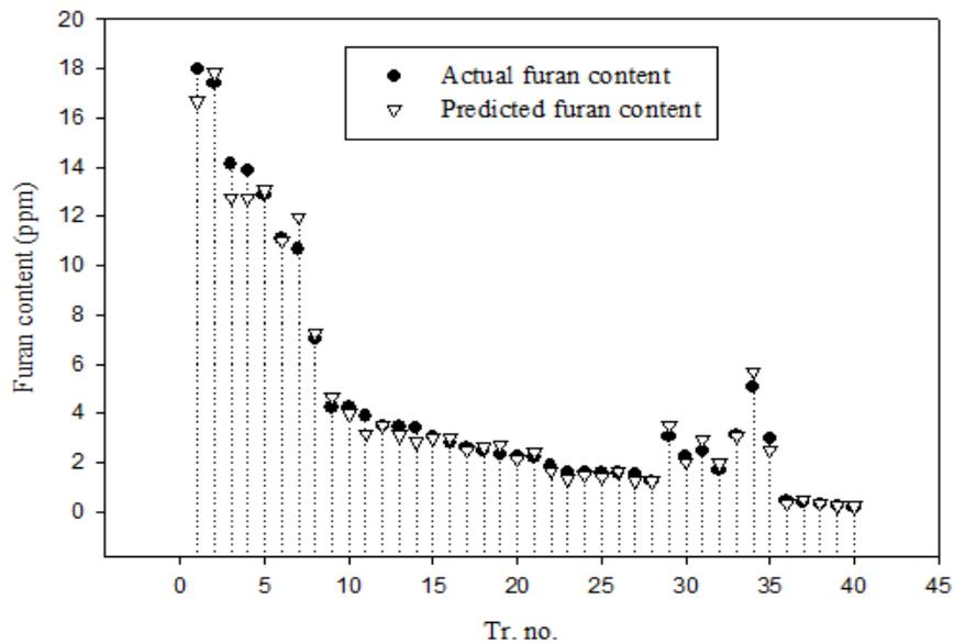
Figure 12: Furan content prediction in transformer oil with CO, CO<sub>2</sub>, acidity and BDV as inputs
