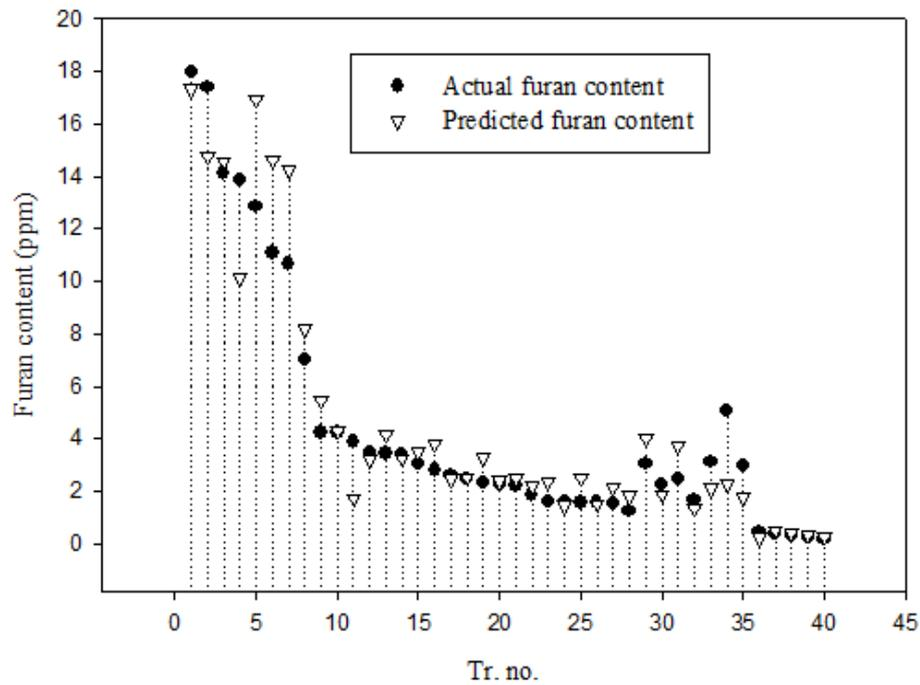
Figure 13: Furan content prediction in transformer oil with CO, acidity and BDV as inputs
