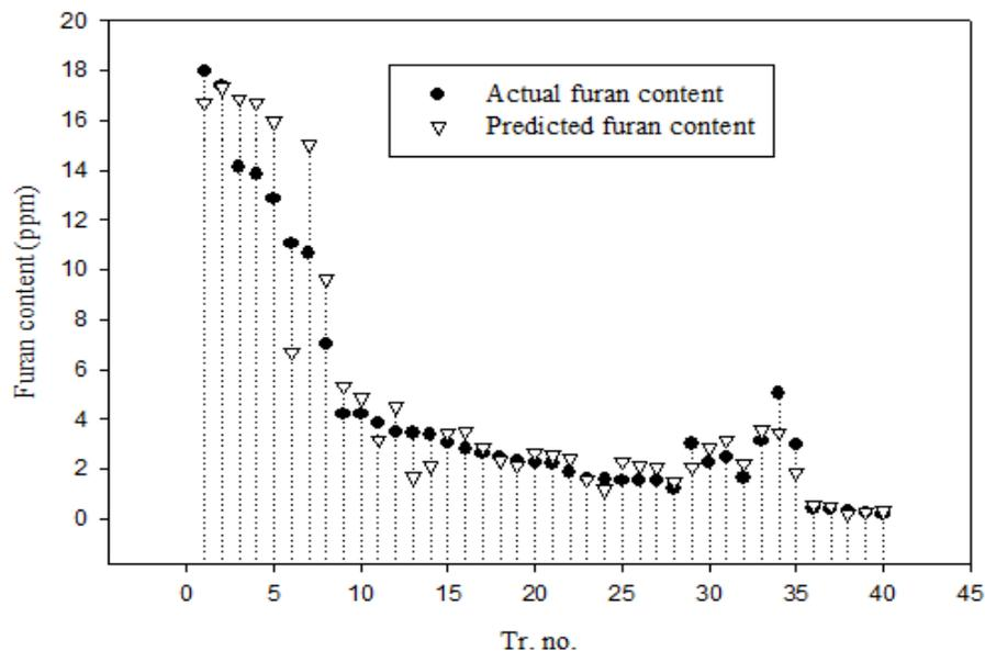
Figure 10: Furan content prediction in transformer oil with CO, TDCG, acidity and BDV as inputs
