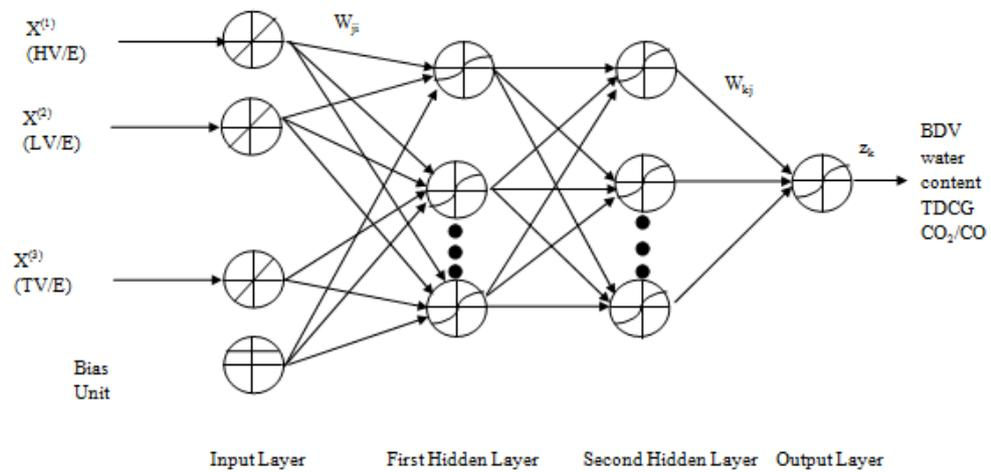
Figure 3 : Artificial neural network structure proposed for predicting BDV, water content, TDCG and  $\text{CO}_2/\text{CO}$
