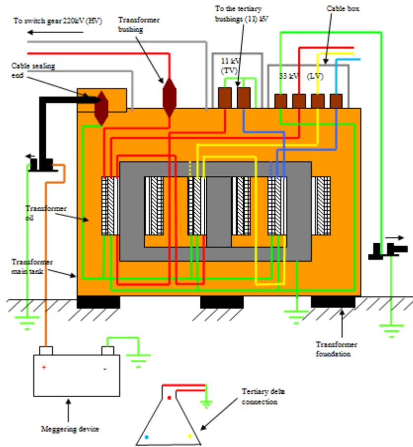
Figure 2: Side view of practical megger test conducted in the site
