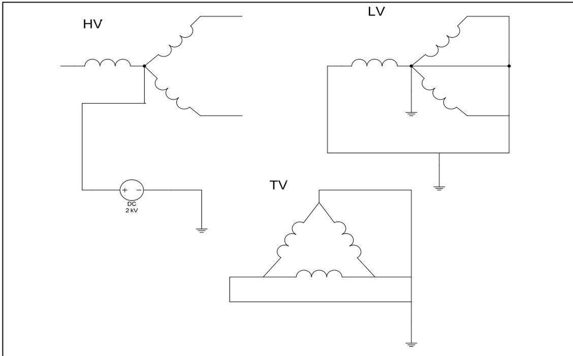
Figure 1: Schematic diagram of Megger test (HV/Ground)
