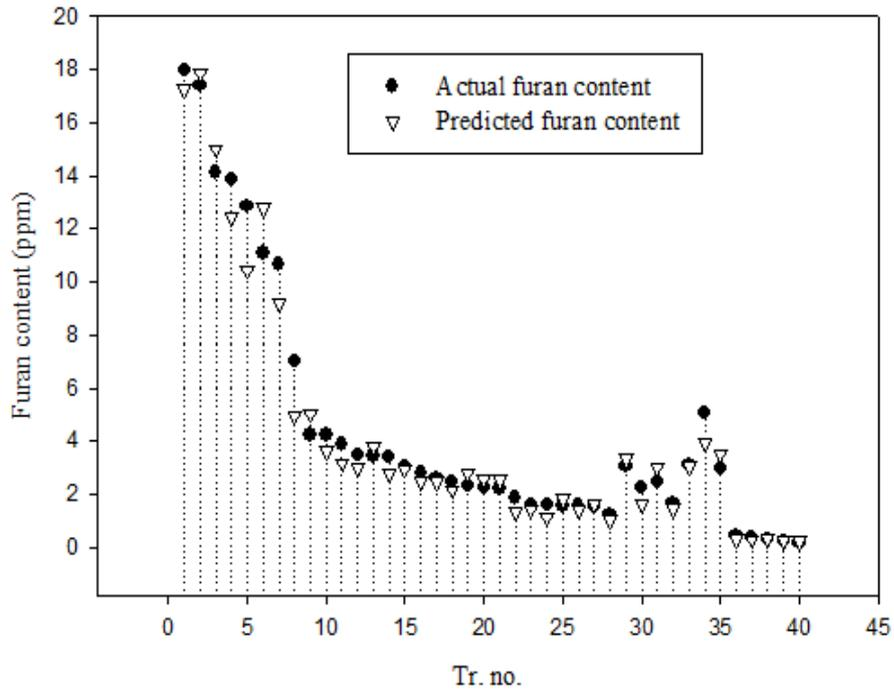
Figure 11: Furan content prediction in transformer oil with CO<sub>2</sub>, acidity and BDV as inputs
