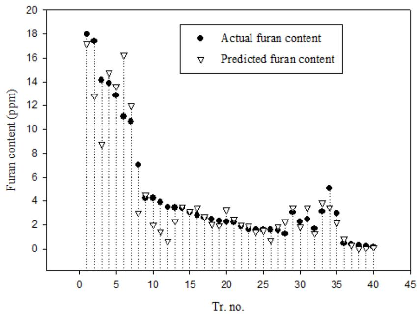
Figure 14: Furan content prediction in transformer oil with TCG, acidity and BDV as inputs
