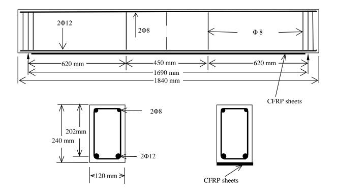
Figure 1. Tested beams details
