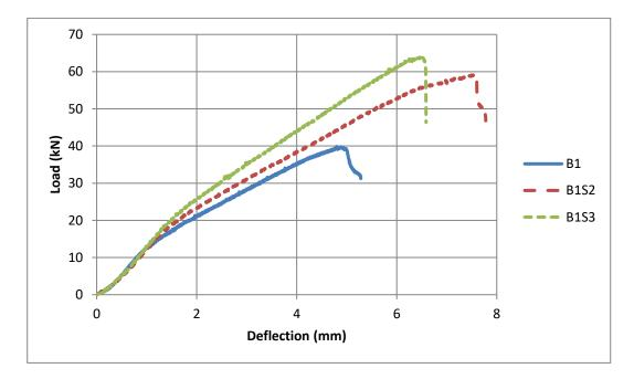
Figure 2. Load versus midspan deflection response
