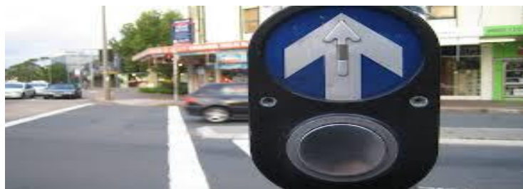
Figure 33 Crossing audio tactile [89].
