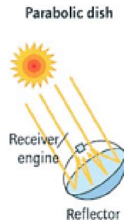
Figure 11: Parabolic Dish Reflector [34]
