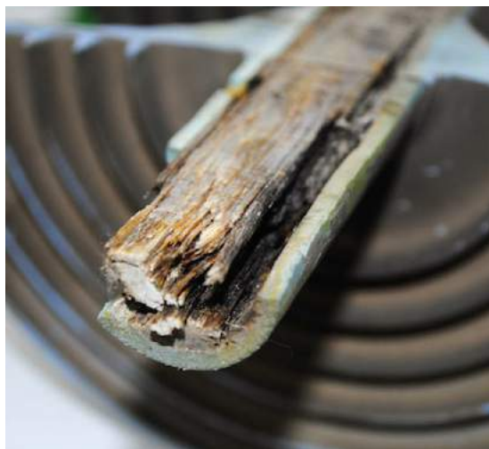
Figure 2.8: Brittle fracture on an insulator [30].
