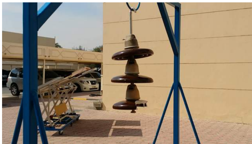
Figure 3.3: Custom built tower for holding insulators.
