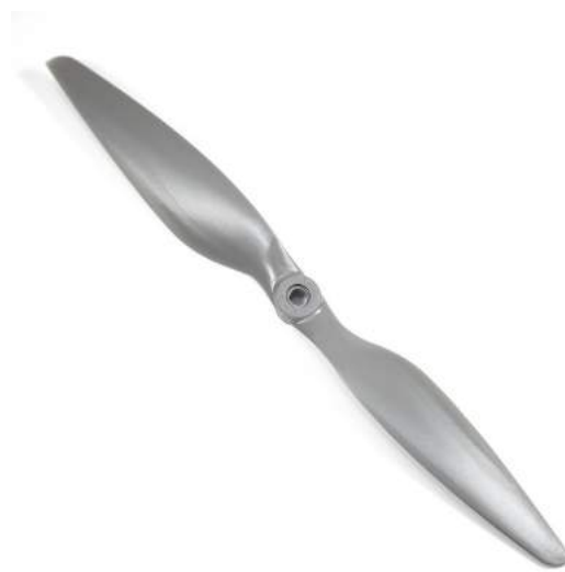
Figure 3.8: A commonly used 16 x 5.5 inch propeller in quadcopters where 16 is the diameter of the propeller and 5.5 is the pitch of the propeller [51].
