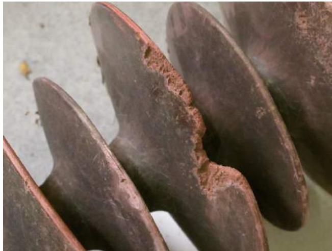
Figure 2.10: Insulator damaged due to birds pecking [30].
