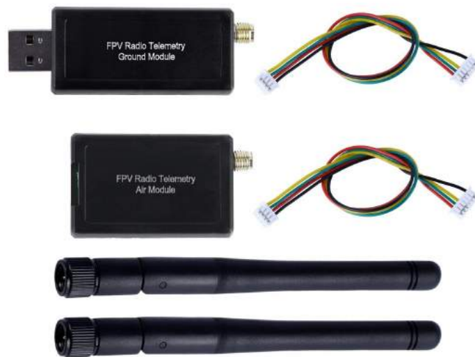
Figure 3.16: A common telemetry device used in quadcopters [61].
