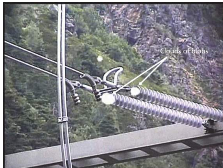
Figure 2.12: “Blob” captured via daylight corona camera [33].
