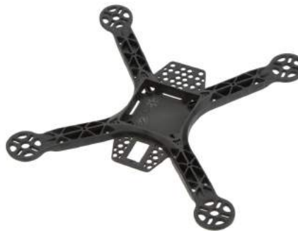
Figure 3.7: An example of a quadcopter frame [48].
