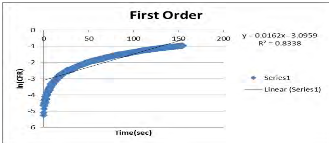
Figure 38: First Order Model plot for the first batch of NH 2 liposomes at a power density of 7.46mW/cm 2 .
