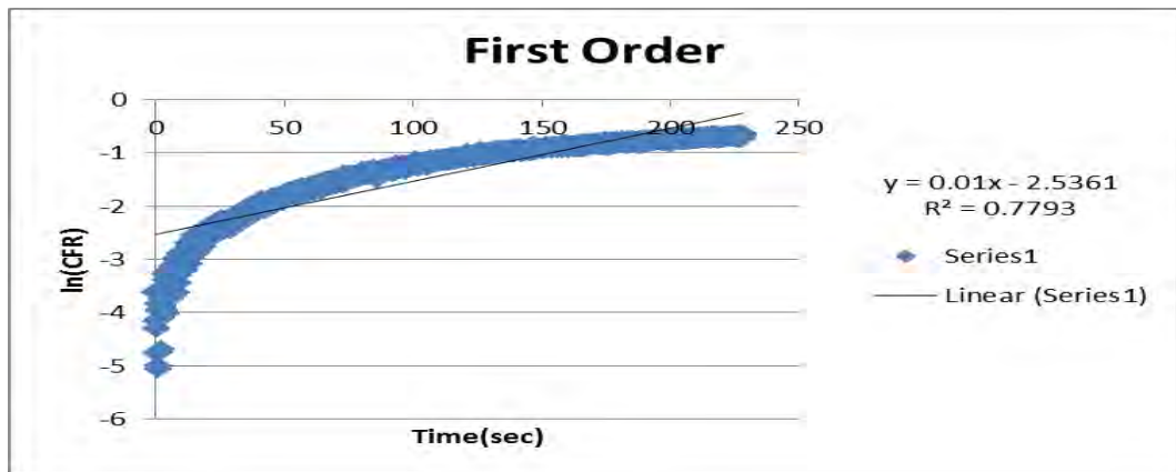
Figure 47: First Order Model plot for the first batch of Tf liposomes at a power density of 7.46mW/cm 2 .
