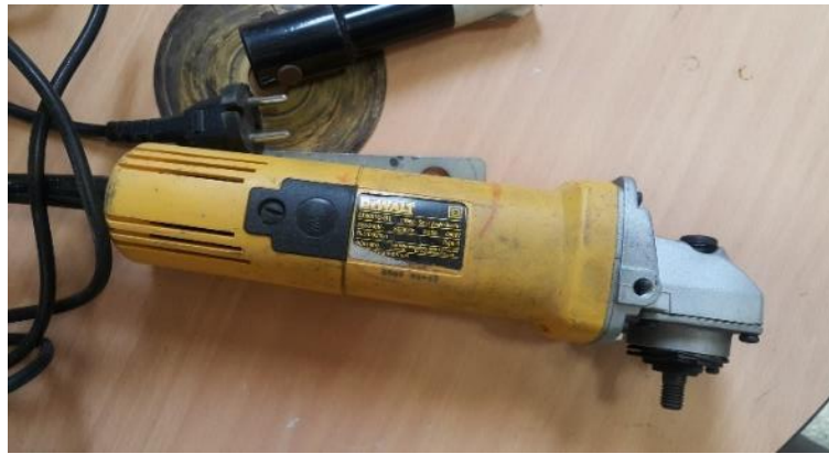
Figure 3.5: Motor used for driving the rotation of the cylinder.
