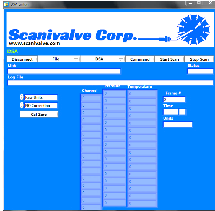
Figure 3.6: DSA LabVIEW software used for collecting pressure data.
