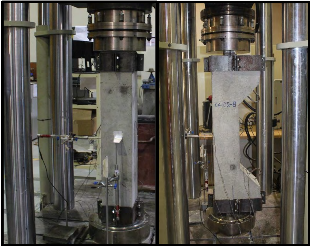
Figure 3.10: Photos of typical test setups for concentric columns (left) and eccentric columns (right)
