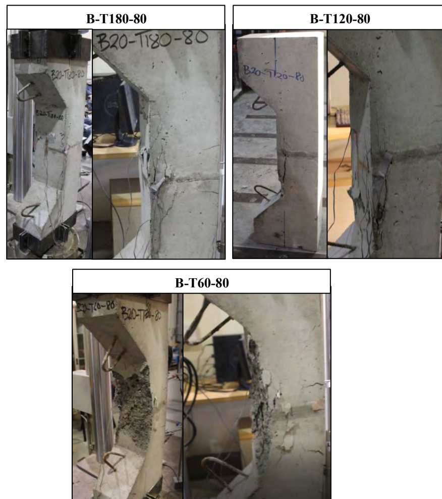
Figure 4.5: Photos of Group 2 column specimens tested under 80 mm eccentricity, after failure
