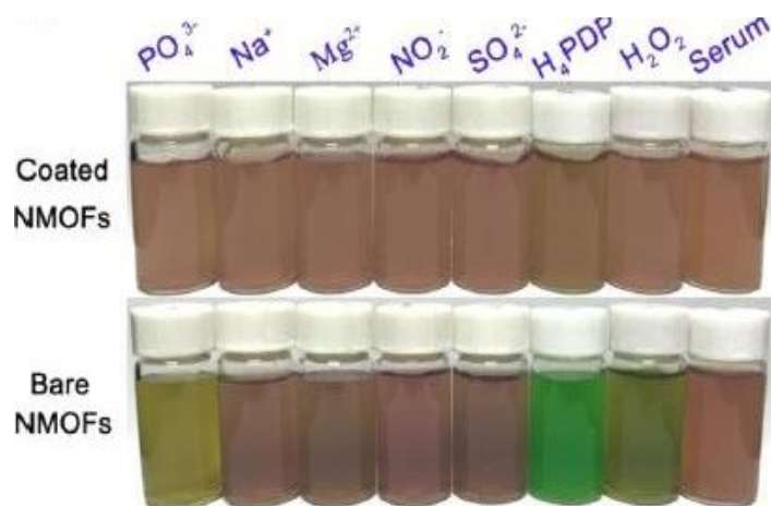
Figure 10: The corresponding photographs illustrating the changes of bare and coated nano Zr MOFs suspensions under various chemical environments (100 mM) or 10% of the above compounds [62].
