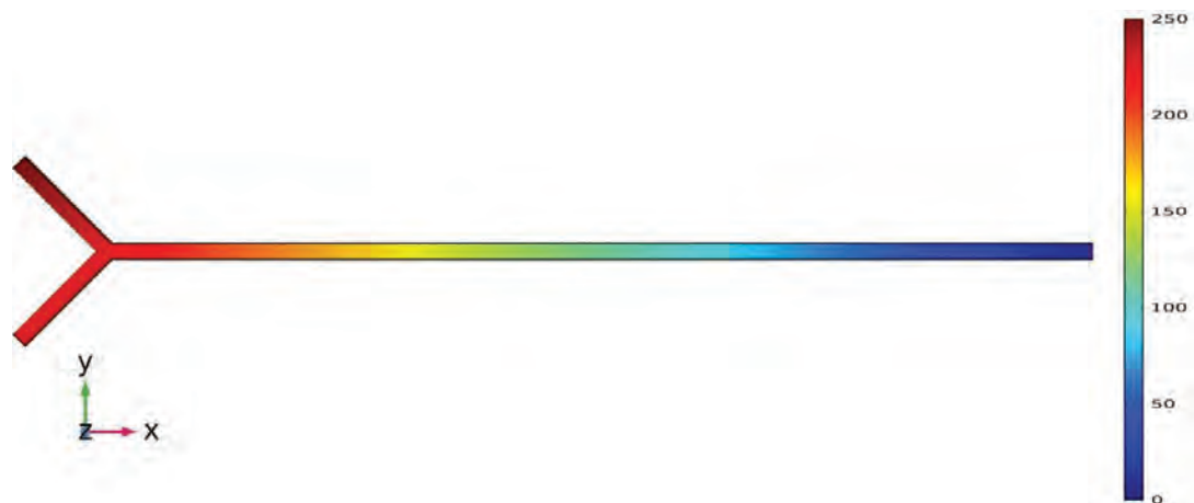
Figure 31 Pressure distribution along the Y-shaped microchannel when the solute is switch on, and the solvent is switched off.
