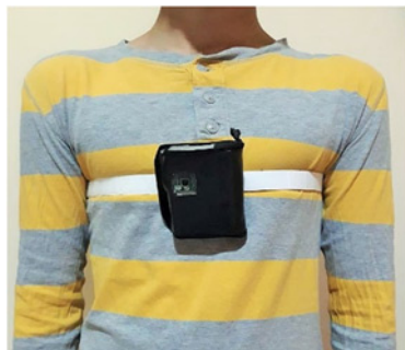
Fig. 6 Wearable Multi-Sensor unit attached to the subject's chest
