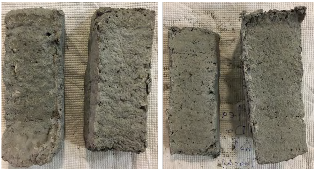
Figure 61: Typical Fractured Interface of Printed Specimens (Left) t = 2.5 hrs and (Right) t = 4 hrs.
