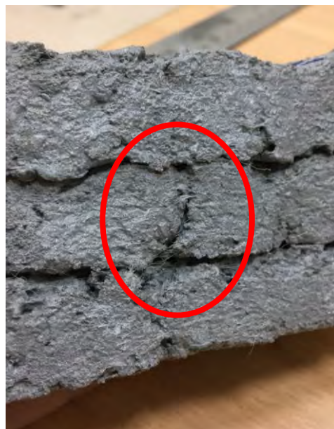
Figure 42: Stoppage in Extrusion Process.
