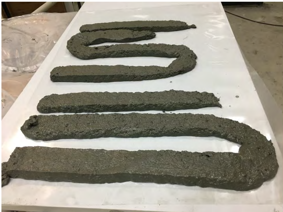
Figure 44: Continuously Printed Filaments for Extrudability Evaluation.
