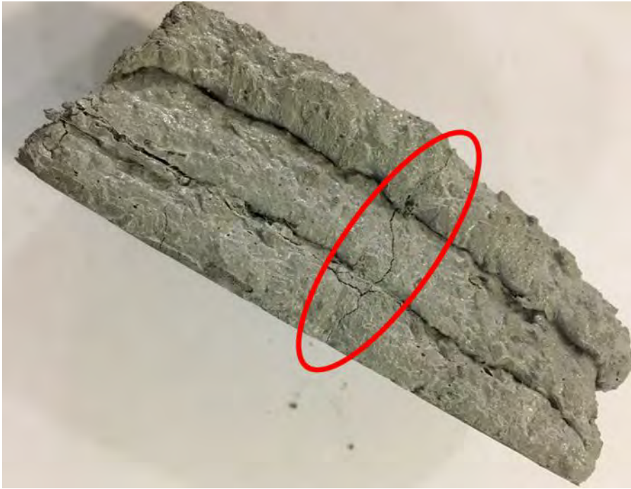
Figure 63: Vertical Crack Along Layers of a Printed Specimen in Bond Test.
