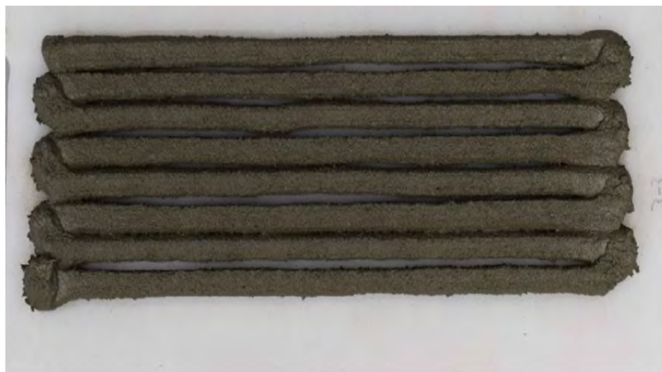
Figure 14: Top View of 2-m long printed mortar strip [22].
