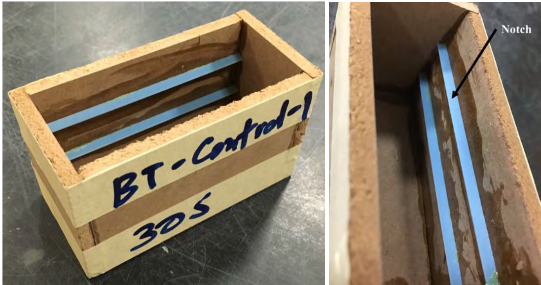
(a) (b) Figure 56: Bond Shear Test Control Specimen (a) Mold and (b) Blow Up.
