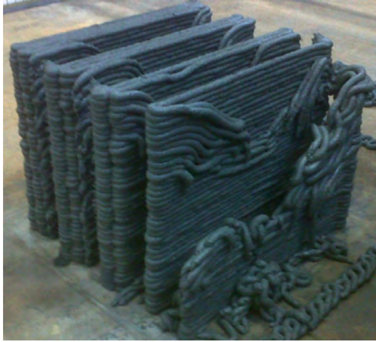
Figure 11: Several printed objects with different number of strips in the horizontal plane [24].
