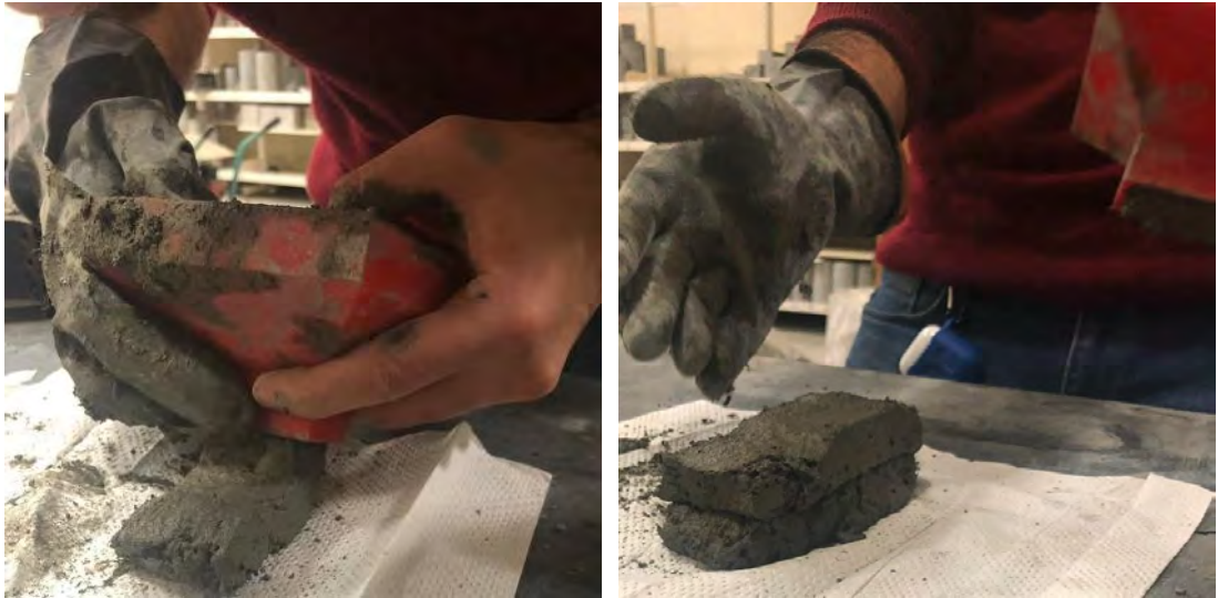
Figure 18: Manual Extrusion, (left) sample extruded concrete, (right) sample layered object.
