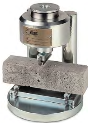
Figure 23: Concrete Prism Under ASTM C348 Flexural Strength Test [54].
