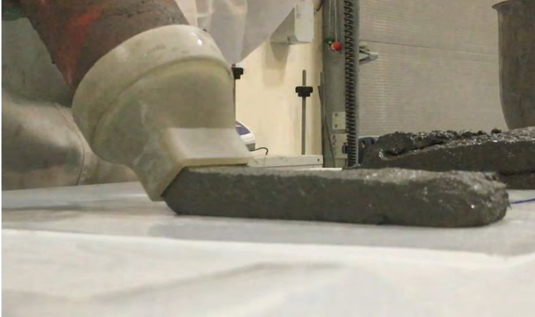
Figure 20: Manual Extrusion using The Injection Tool.
