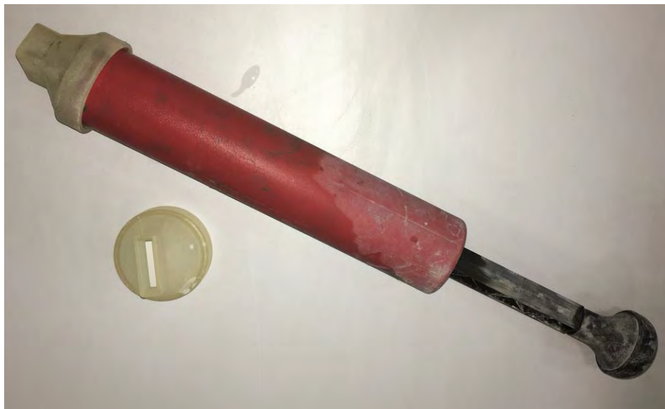
Figure 19: Injection Tool and Fitted Nozzle for Extrusion.
