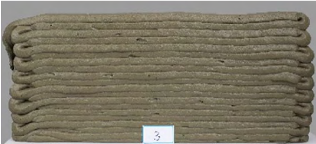
Figure 10: Elevation of Mortar Layers Printed for the Evaluation of Buildability [22].
