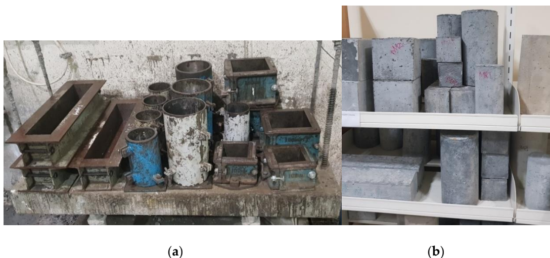
Figure 4. Samples preparation for mechanical properties. (a) Molds used for sample preparation, (b) Samples for mechanical evaluation.
