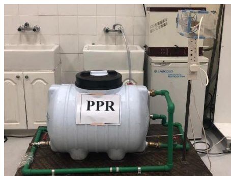
Figure 3: PPR pipe loop system
