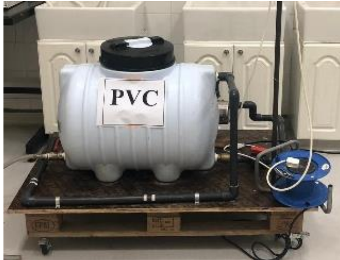
Figure 5: PVC pipe loop system
