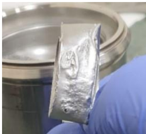
Figure 17 Sample affected by high energy coating at 800 rpm
