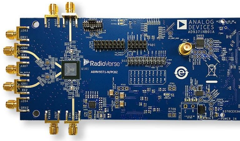
Figure 4.5: ADRV9371 2x2 MIMO evaluation board
