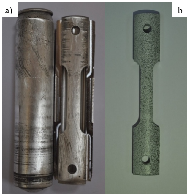
Figure 10: a) shows the extruded tube and after its CNC machined b) dumbbell specimen
