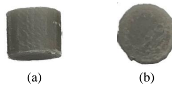
Figure 4.2: 3D printed PLA-SiC compression sample (a) side-view and (b) top-view.
