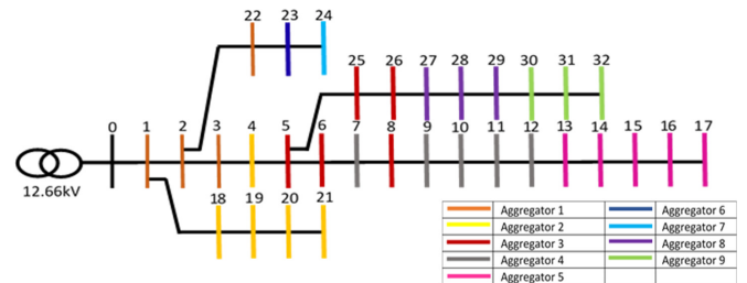
Fig. 3. IEEE 33 bus system load buses divided among nine aggregators [28]
