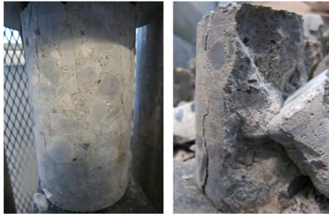
Fig. 9. Views of tested WG concrete cores extracted from recycling center.
