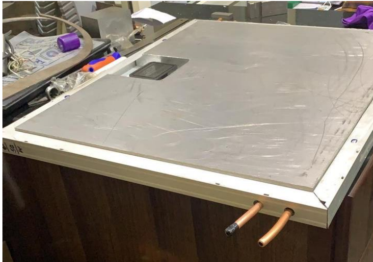
Figure A-2: Rear-side of the PVT system
