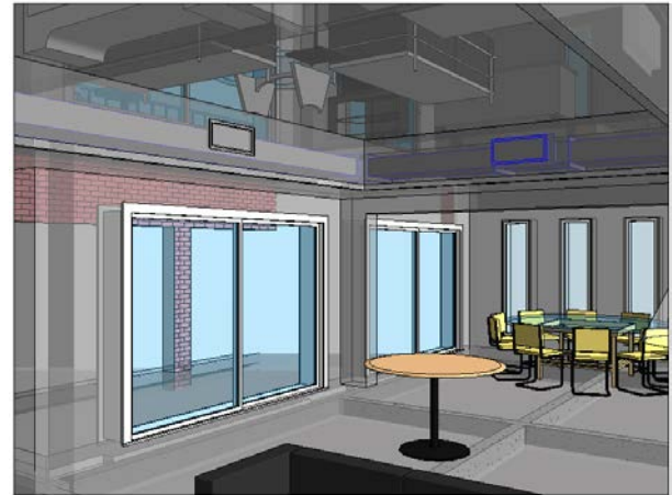
Figure 5. A pre-arranged view to allow seeing the HVAC grilles in the ceiling of the living room (transparency mode).
