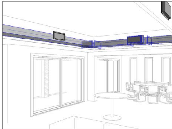
Figure 4. A pre-arranged view to allow seeing the HVAC grilles in the ceiling of the living room (shaded HVAC elements mode).
