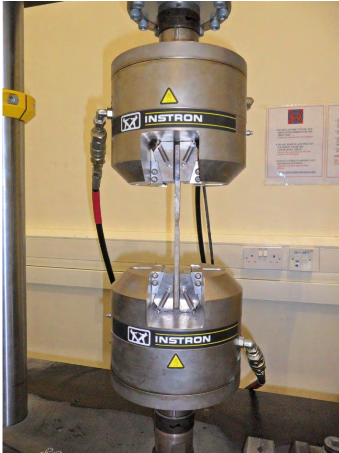
Steel Coupon test
