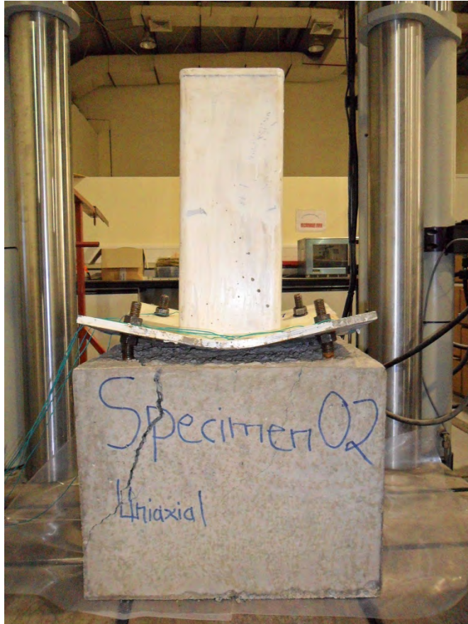
Base Plate at Failure
