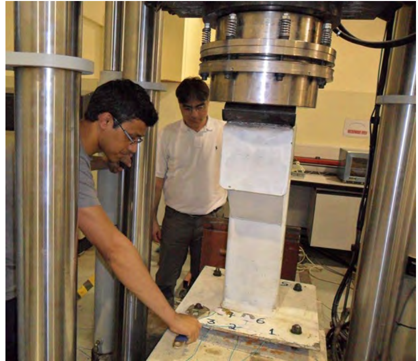
Final adjustment of base plate
