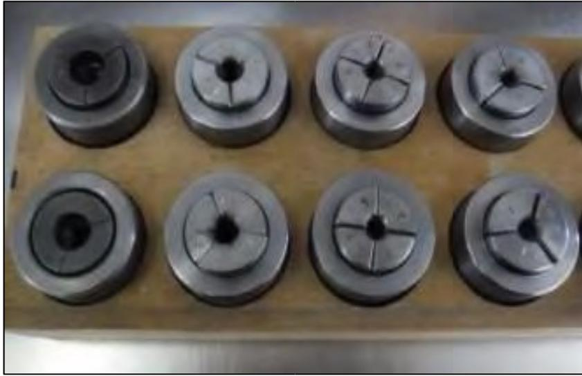
Figure 4.8: Steel Grips for Gripping Both Ends of GFRP Bars during the Uniaxial Test
