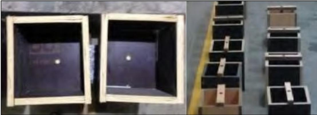
Figure 3.1: Samples of Cubical Wooden Forms Prepared for the Pullout Test
