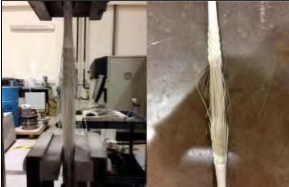
Figure 5.9: GFRP Bar Mode of Failure after a Tensile Test
