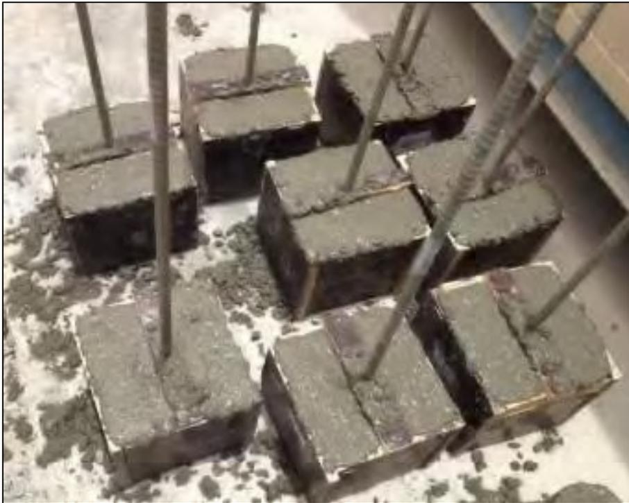
Figure 4.4: Samples after Casting
