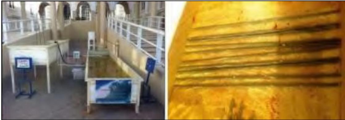
Figure 3.3: AUS Sustainability Center for Simulating the Splash Zone
