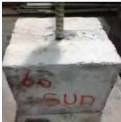
Figure 5.2: Failure of the Concrete Cover
