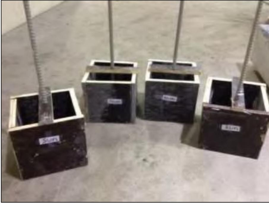
Figure 4.3: Samples of Cubic Wooden Forms Prepared before Casting Concrete
