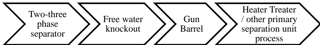
Figure 5: Pretreatment of produced water [19]
