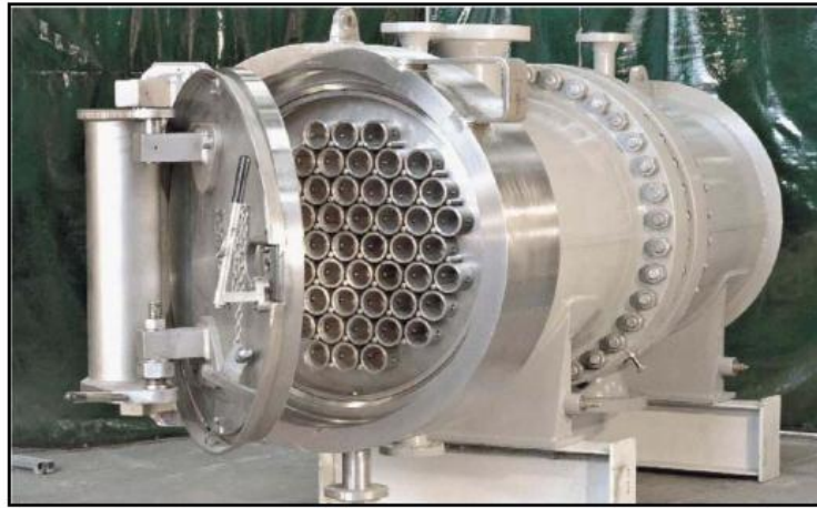
Figure 4: A vessel containing multiple hydrocyclones for de-oiling of produced water with maximum capacity – 120,000 barrels/day [10]
