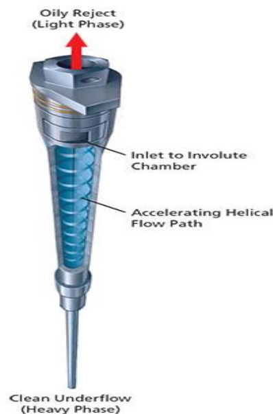
Figure 3: Schematic diagram of de-oiling hydrocyclone [13]
