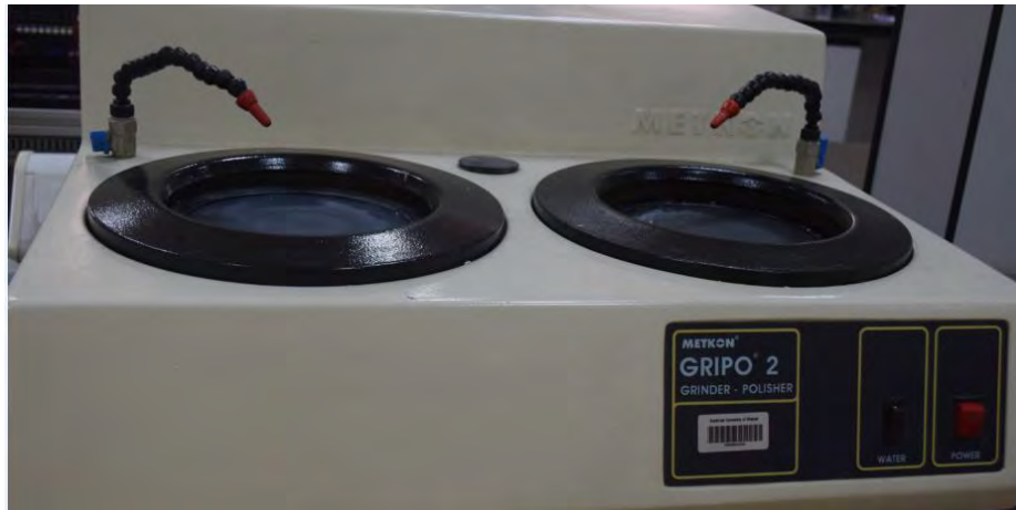
Figure 25: Sample grinding machine.
