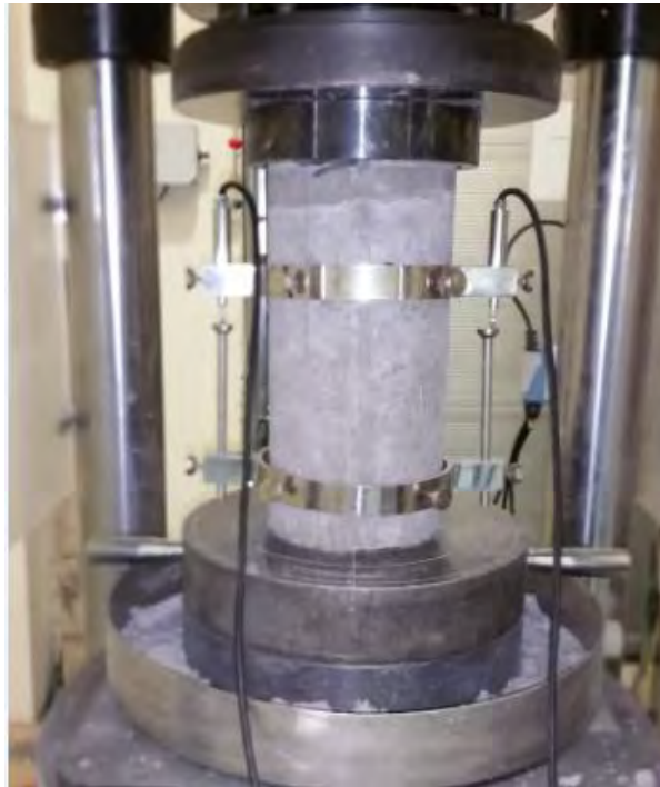
Figure 19: Modulus of elasticity test setup.
