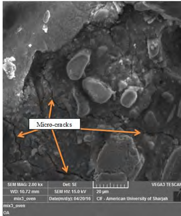
Figure 49: SEM image for oven cured G100 specimen.
