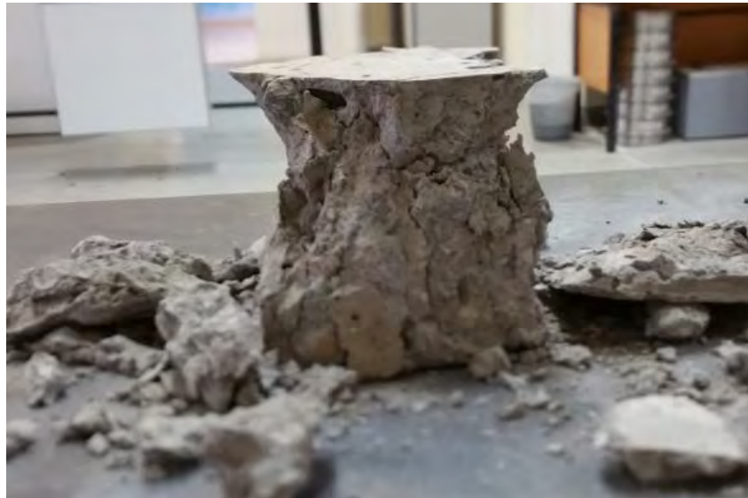
Figure 29: Failure shape of geopolymer concrete cube under compression.
