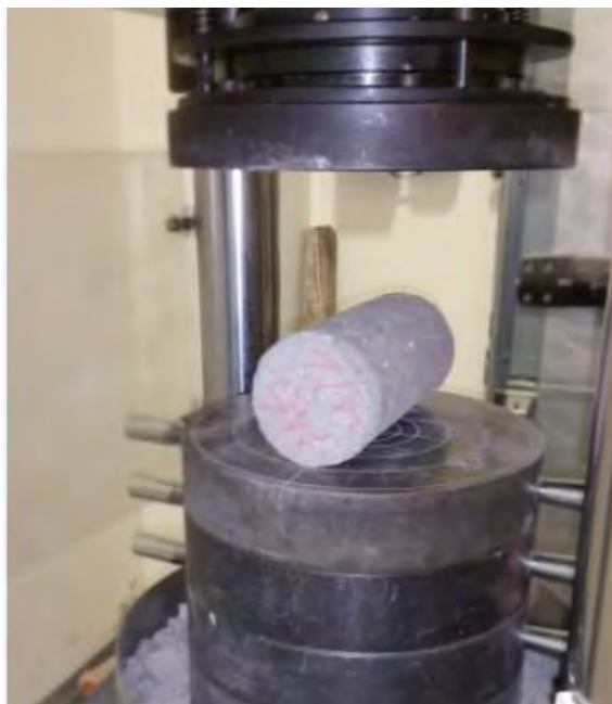
Figure 16: Tensile strength test setup.
