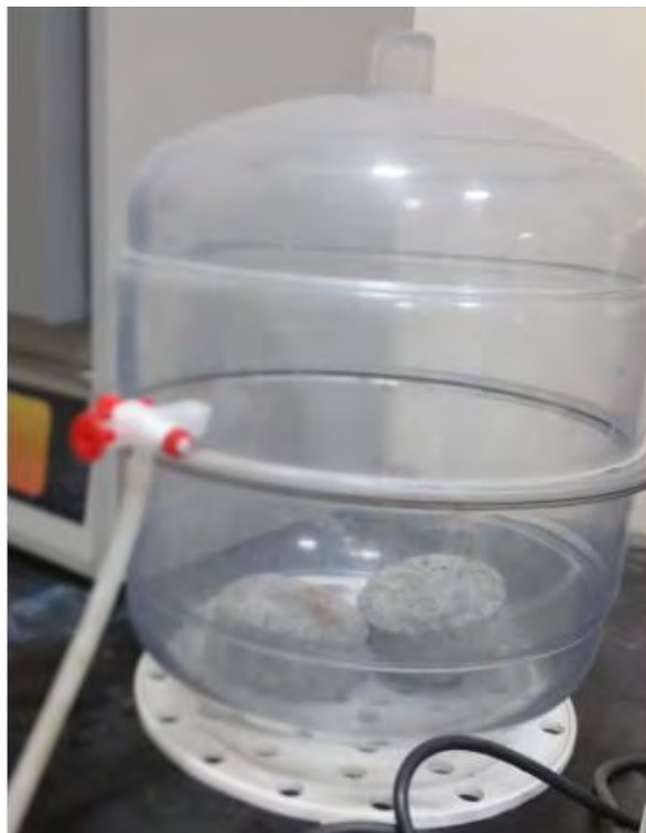
Figure 20: RCPT samples incubated in vacuum chamber.
