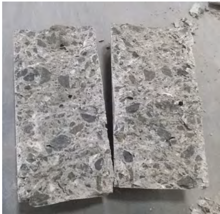
Figure 32: Failure of geopolymer concrete cylinder under tensile test load.
