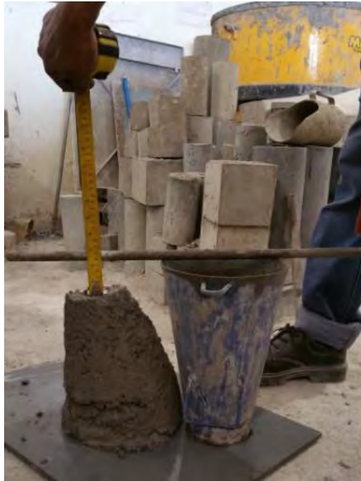
Figure 13: Slump test setup.
