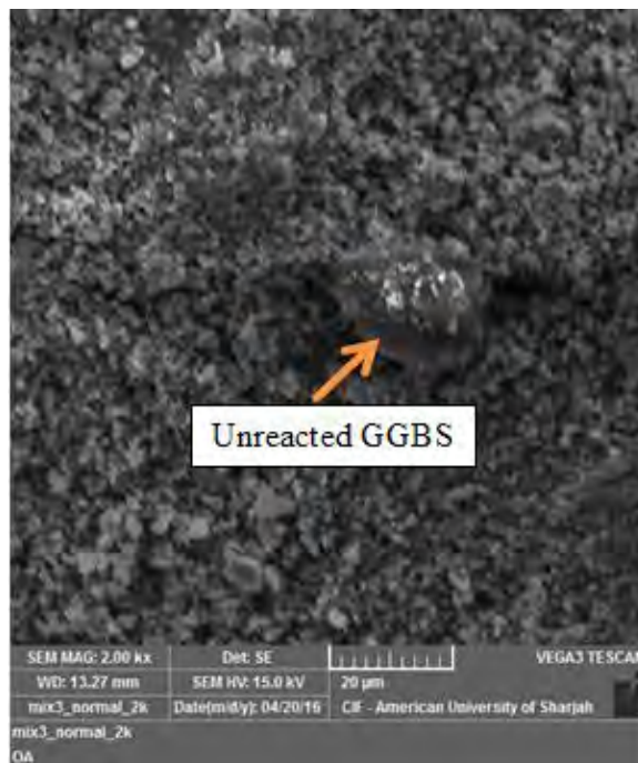
Figure 44: SEM image of ambient cured mix G100 specimen at 28 days.
