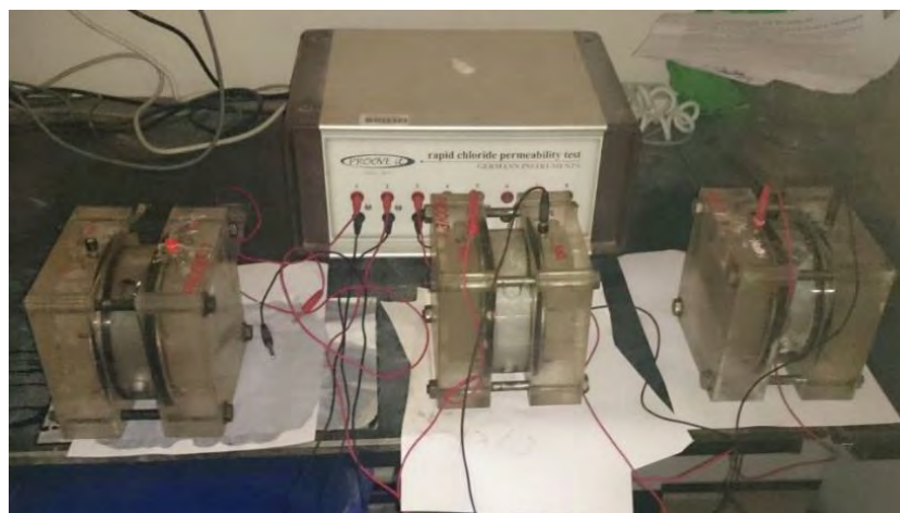
Figure 22: RCPT computerized system.
