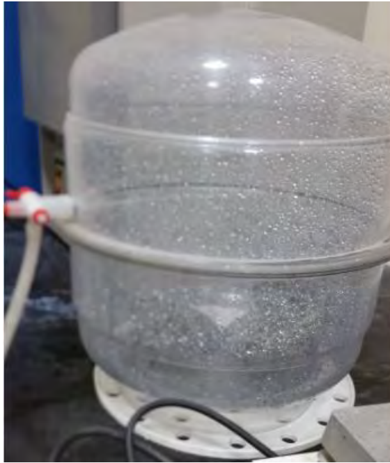
Figure 21: Distilled water going inside vacuum chamber due to pressure difference.
