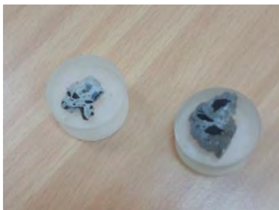
Figure 24: Concrete thin sections prepared for SEM with plastic coating.
