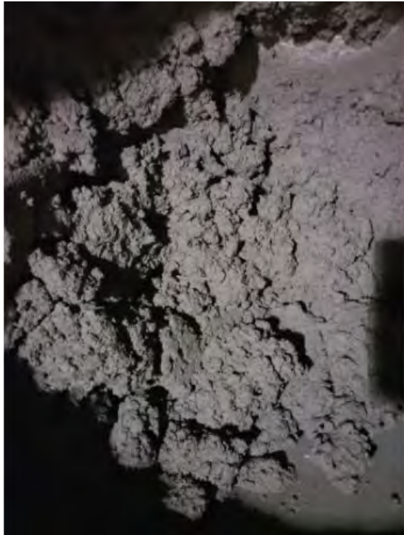
Figure 27: Very stiff geopolymer mix F15-G70-S15.
