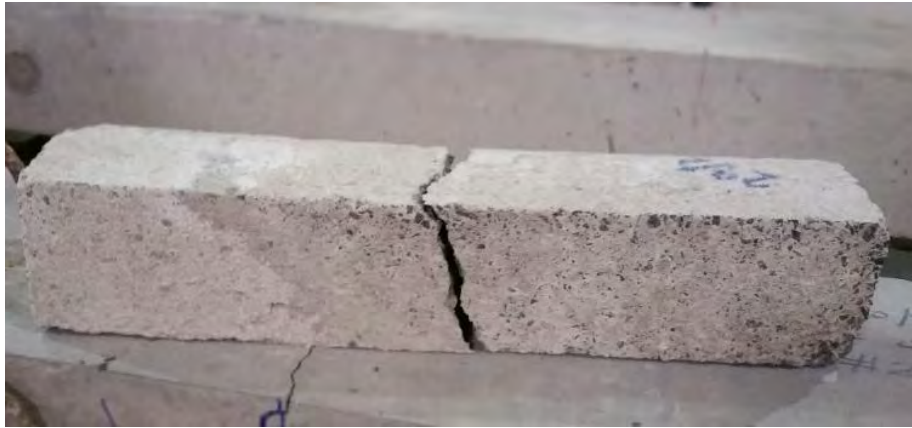
Figure 35: Failure of geopolymer concrete beam after flexural strength test.
