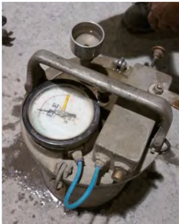
Figure 14: Air content test apparatus.
