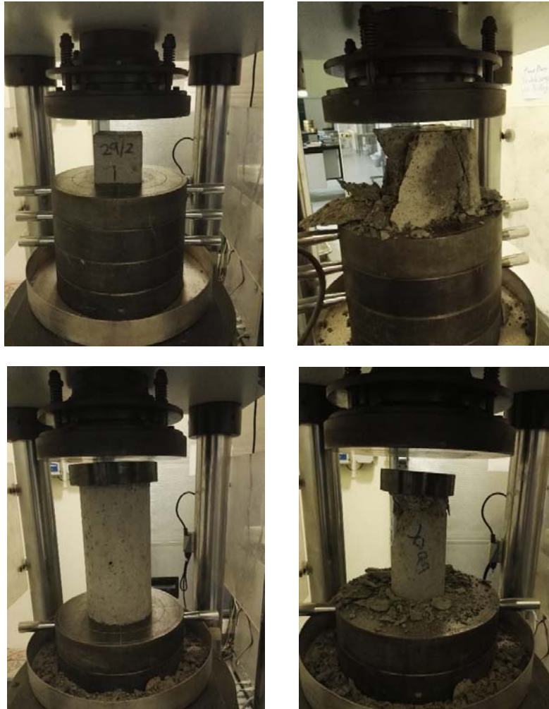
Figure 3.4: Compressive strength test.
