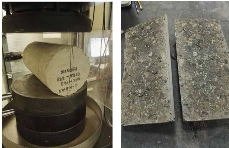
Figure 3.6: Splitting tensile strength test.
