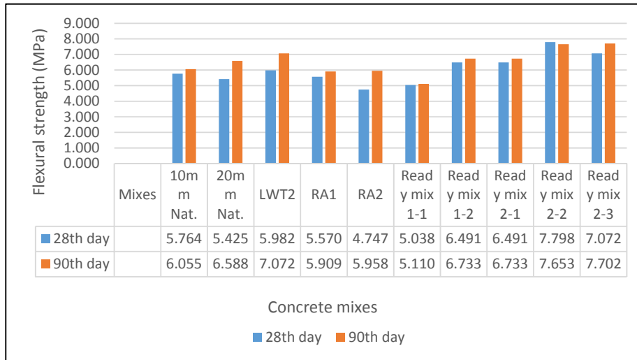
Figure 4.7: Flexural strength for different concrete mixes at 28 th and 90 th day.
