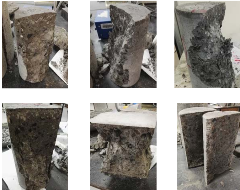
Figure B.9: Compressive strength failure for C80 ready-mix concrete
