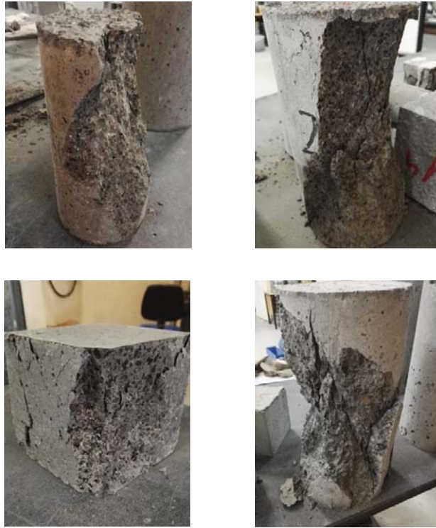
Figure B.4: Compressive strength failure for LWT2 concrete mix
