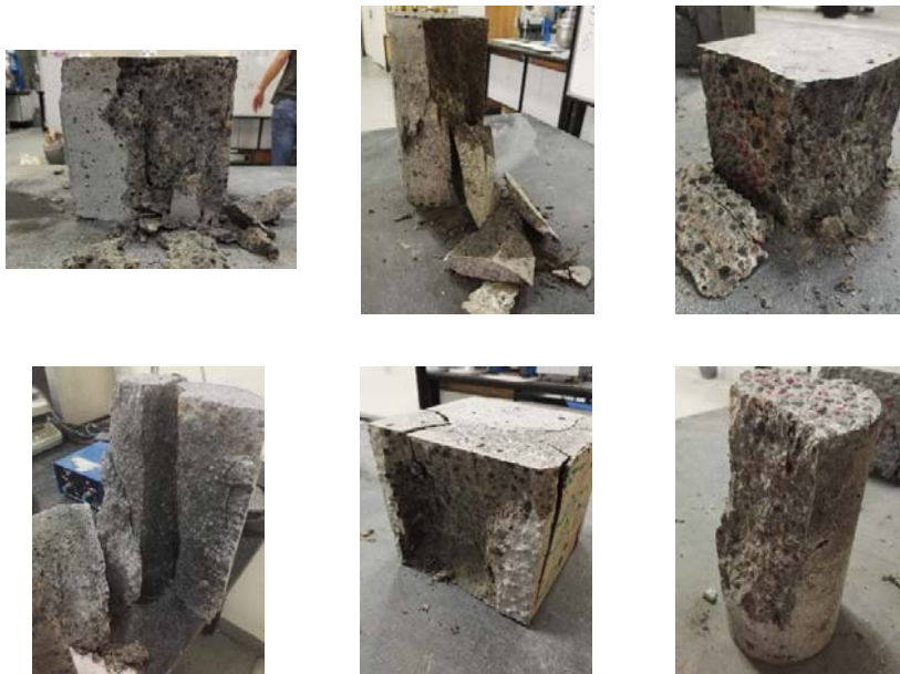
Figure B.3: Compressive strength failure for LWT1 concrete mix
