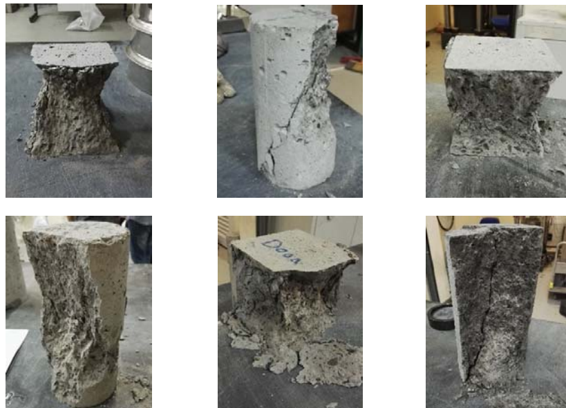
Figure B.1: Compressive strength failure for 10 mm Natural concrete mix
