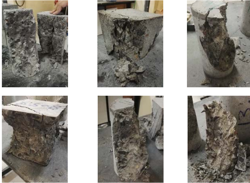
Figure B.2: Compressive strength failure for 20 mm Natural concrete mix
