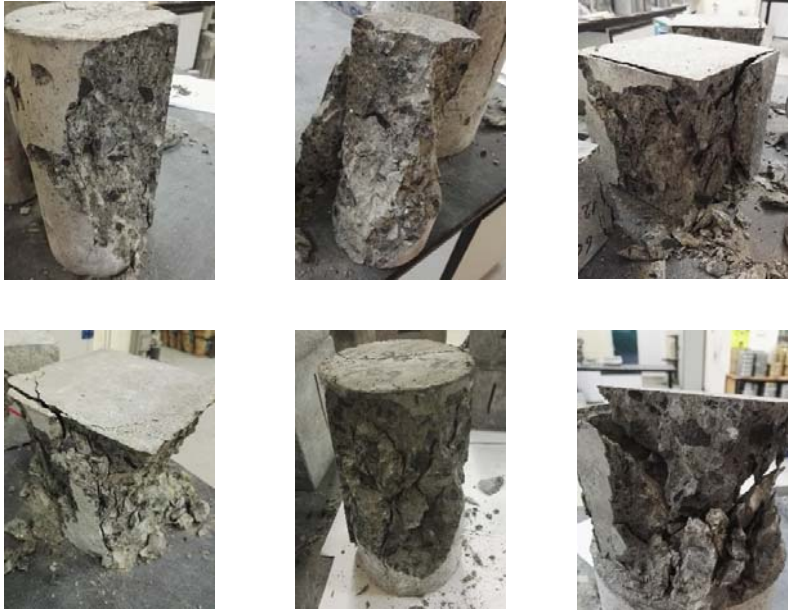
Figure B.8: Compressive strength failure for C60 ready-mix concrete
