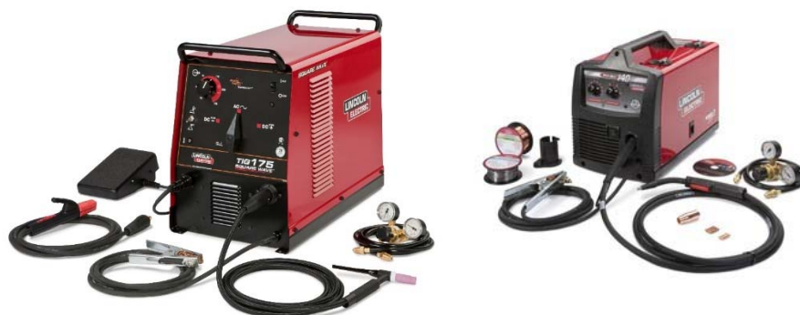
Figure 16: GTAW tool (left) [48] and GMAW tool (right) [49]
