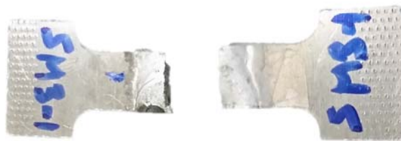
Figure 25: Tensile test specimen after testing
