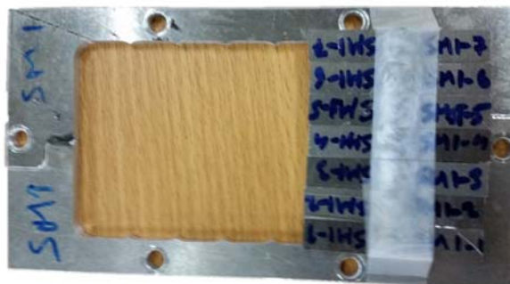
Figure 27: Welded plate toughness specimens cut
