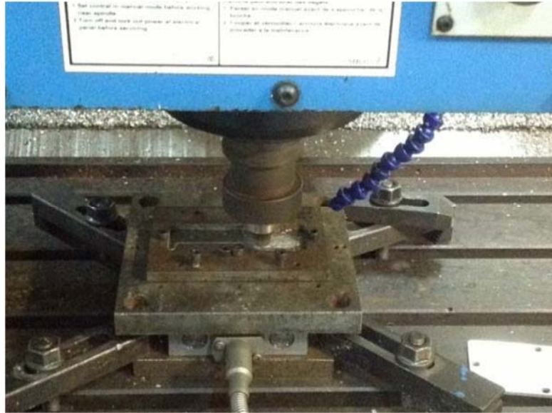
Figure 17: FSW welding tool in CNC milling machine [50]
