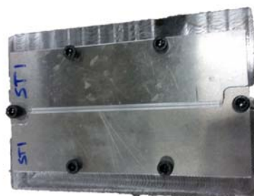
Figure 15: Plates fixed on weld backing jig
