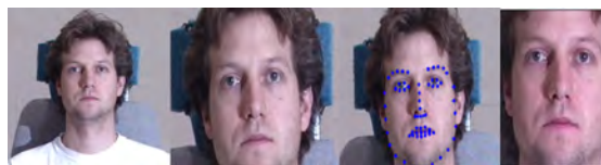
Figure 4: Input image with face is used to extract face, calculate facial landmarks which are used to align, extract and scale face to pre-defined parameters
